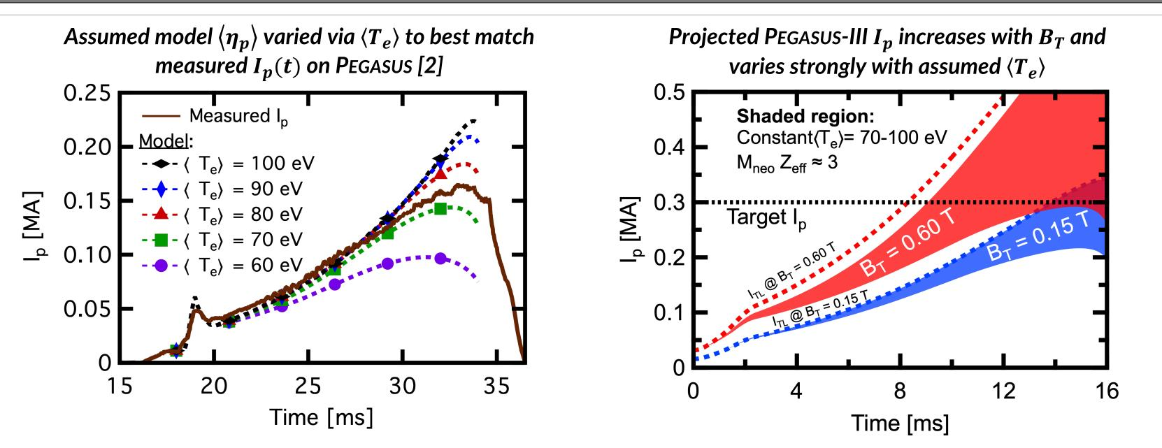
Reliable  $I_p(t)$  projections require a model to scale helicity dissipation
