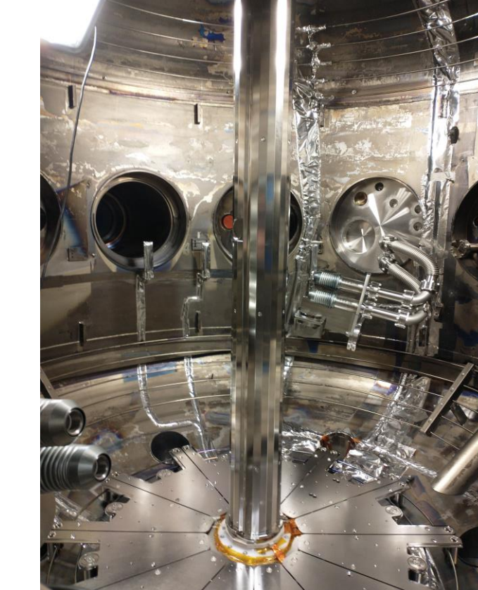
Interior of vacuum vessel showing new vacuum wall covered in core armor and new LHI hardware
