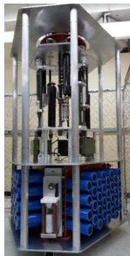
Klystrons powered by new DC-DC resonant supplies
