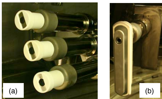
Fig. 6. (a) 3-arc source array with individual slotted electrodes; (b) arc source with large area electrode, floating Mo backing plate, and scraper limiter.
