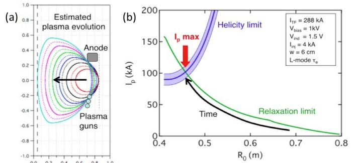
Fig. 1. (a) Geometric evolution with midplane startup. (b)  $I_p$  evolution with helicity and relaxation limits.
