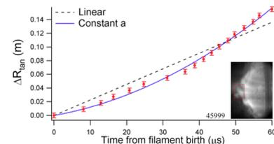
Fig. 7. Radial propagation and acceleration of peeling filament.
