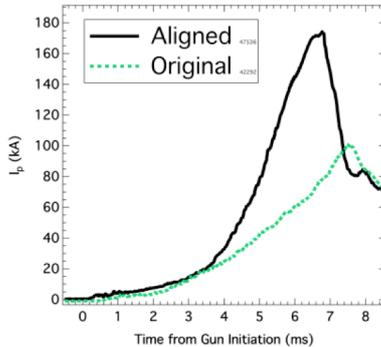
Fig. 3  $I_p$  for aligned ( $w \approx 2$  cm) & original gun structure ( $w \approx 6$  cm).
