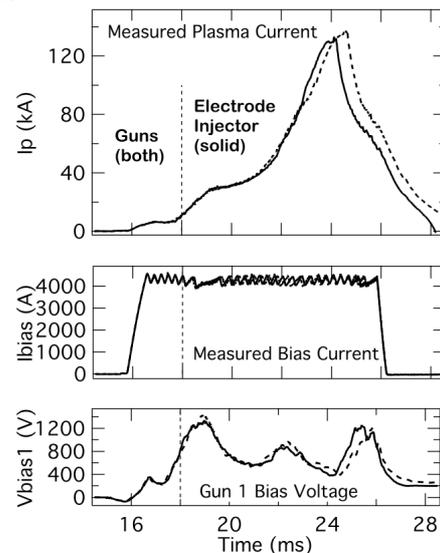
Fig. 5. Arcs off @18 ms;  $I_p$  growth by passive electrode (solid). Full-arc-on traces (dashed) shown for comparison.
