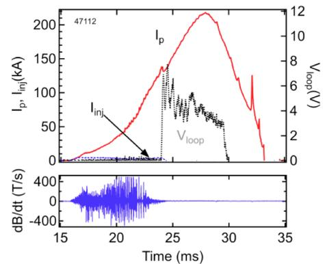
Fig. 4. (a) HI target coupled to ohmic drive; (b)  $n=1$  mode activity.
