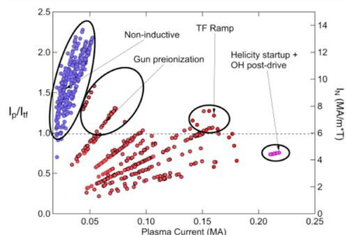
Fig. 6.  $j(r)$  modification techniques allow achievement of high  $I_p/I_{TF}$ .
