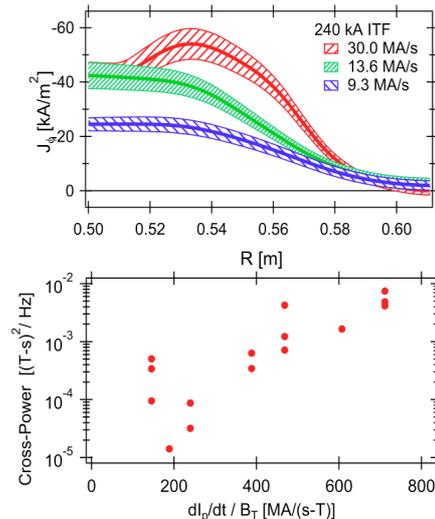
Fig. 8. (a)  $j_{\text{edge}}(R)$  variation with  $dI_p/dt$ ; (b) Peeling EM fluctuation power increasing with  $j_{\text{edge}}/B$ .
