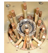
High-Stress OH Solenoid 12-turn TF Bundle
