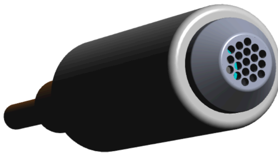
Perforated electrode (no plasma arc) with beveled edge to avoid electrode-BN arcing
