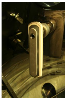
Single arc source with integrated large-area passive electrode
