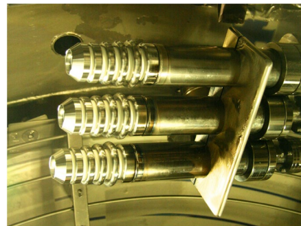
Advanced “Kama” Injector in PEGASUS-III
